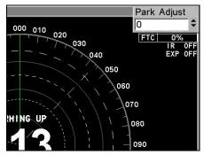
Selecting Adjust Antenna Park will place a dialog box in the upper right-hand corner of the screen. Use Arrow keys to adjust it.
